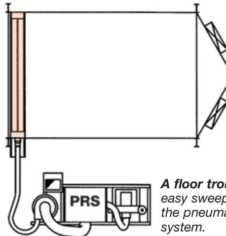
**A floor trough** permits easy sweep-in delivery to the pneumatic-recovery system.
