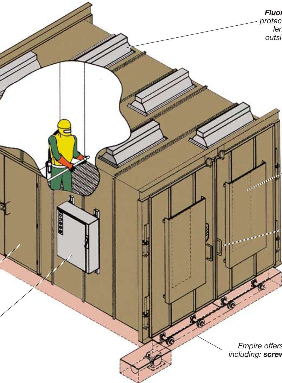
**Fluorescent lighting** on ceiling and sidewalls, protected by clear lexan panels, provides excellent illumination and easy maintenance from outside the blast room. Optional **metal-halide lights** are available for larger rooms.
