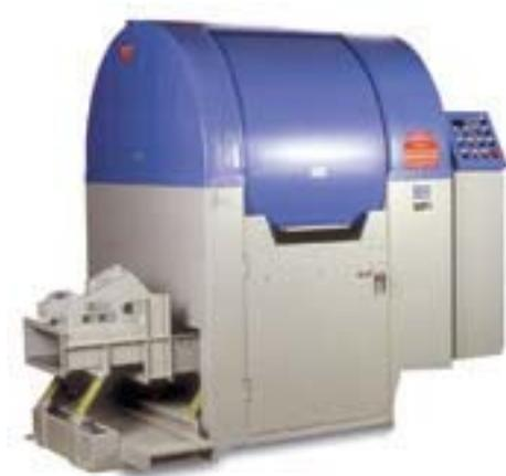
The centrifugal barrel machine has enclosed urethane-lined barrels mounted on a turret. As the turret rotates one direction the barrels are belt or gear driven to rotate to a given ratio in the opposite direction. The individual barrels are loaded with the media, parts to be processed, water and compounds. The action within the barrel is a compressive sliding action creating the maximum energy available today in mass finishing.
