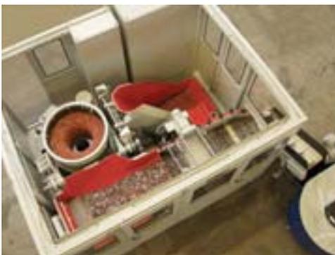
The centrifugal disc is a stationary urethane lined bowl with a rotating bottom urethane lined disc that accelerates the media outward to the sidewall which then decelerates and moves inward to the center of the disc for reacceleration. This change in acceleration and deceleration of the media creates a flowing action over the part, generating energy up to 15 times faster than vibratory with
