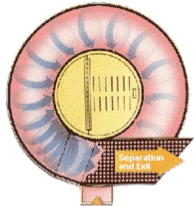
The most significant advantage of a bowl over a tub is that ramps, gates and screens can be added to the bowl allowing self unload of the parts away from the media and out of the machine.
