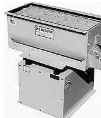
magnets. The tub vibratory machines were developed in the mid 1920s and were a welcome improvement over the rotating barrels that were in production prior to the tubs inception.
