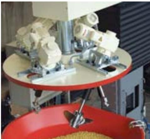
Drag machines are bowl machines that utilize light vibration with fixtures holding and dragging the part thru a heavy mass.
